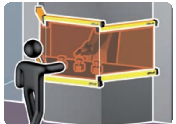
Example of series connection of one master and two slave light curtains for the protection of three sides of the machine
