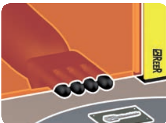
The protected area extends until the light curtain end maintaining the resolution
